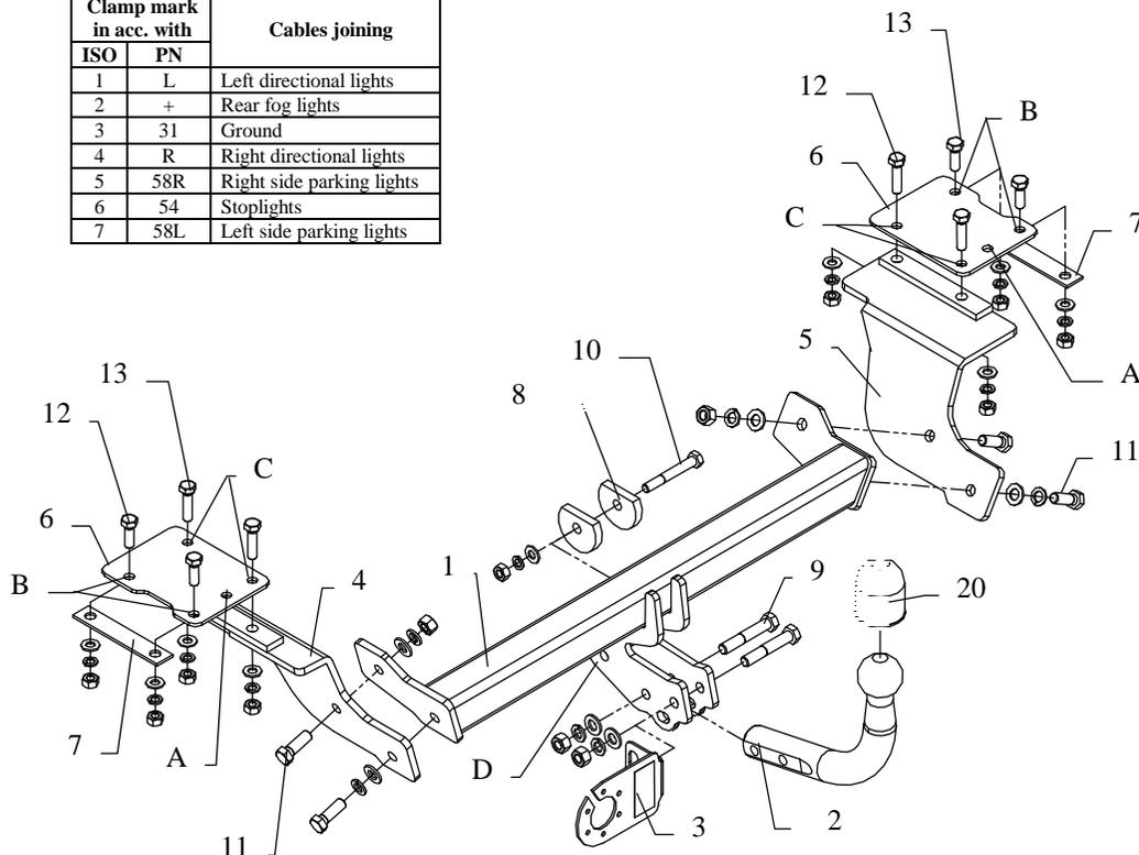
This towbar is designed to assembly in following cars: **SUZUKI SWIFT 3-5 doors**, produced since 1989 till 09.1996 and since 10.1996 till 2003, catalogue number **W13** and is prepared to tow trailers max total weight **1000 kg** and max vertical load **50 kg**.
